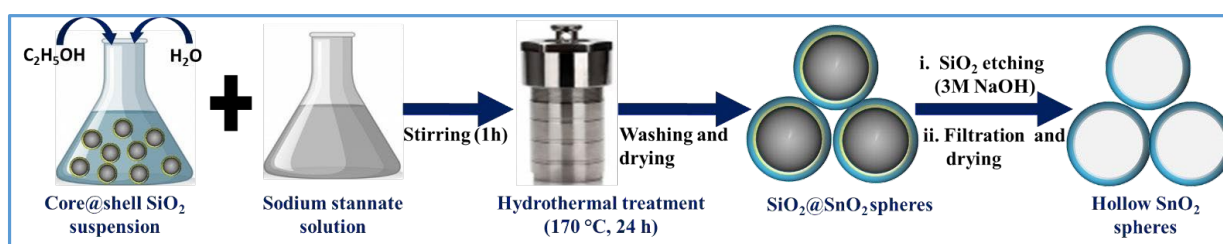
Scheme 1: Synthesis of hollow \text{SnO}_2 nanostructures.
